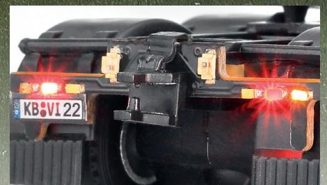
Tail/braking/flashing lights and reverse lights, Infrared transmitter
