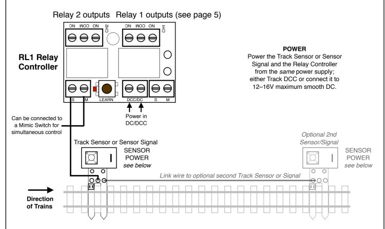
Using one Track Sensor or Sensor Signal the relay will close as soon as the train passes it and then open again about 7 seconds after the last part of the train has passed the sensor. However if you use a second Track Sensor/Signal and link it to the first as shown above, then the relay will close as the train passes the first sensor but not open until the train passes the second sensor, so in this way you can make something operate while a train is located in a particular section of track.
