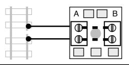
Note that ABC loco decoders must be configured using the instructions from the decoder manufacturer. Some require ABC diode modules to be connected a particular way round, so be sure to carefully follow instructions.
